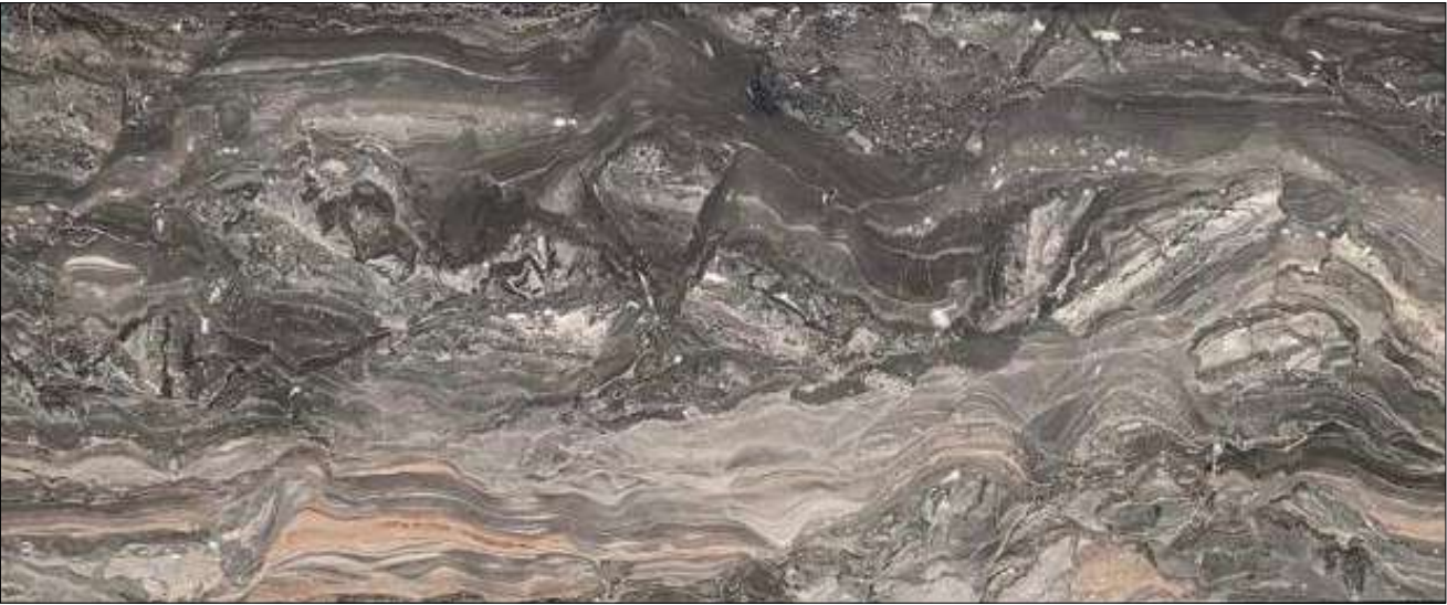
GRIGIO OROBICO The Arabescato Grigio marble is a sedimentary arenaceous lithotype textured with fine-grained gray colored overall. The resistance of this marble to low temperatures, makes it perfect for outdoor paving and covering and indoor use.
